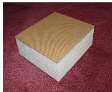
Figure 5. Sandwichpanel with Sizopreg® decking and BioFoam® core
